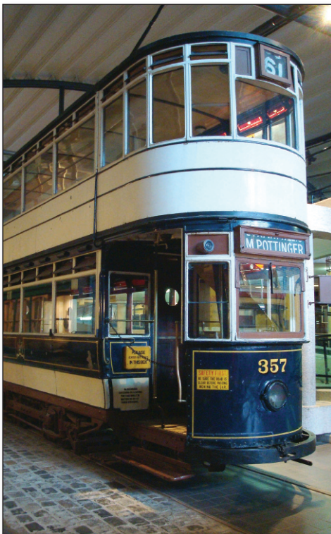
Belfast double decker No 357, was manufactured in 1930 and is now an exhibit inside the Ulster Folk & Transport Museum. The Belfast Corporation Tramways lines were electrified in 1905 and the last tram ran in 1954.
