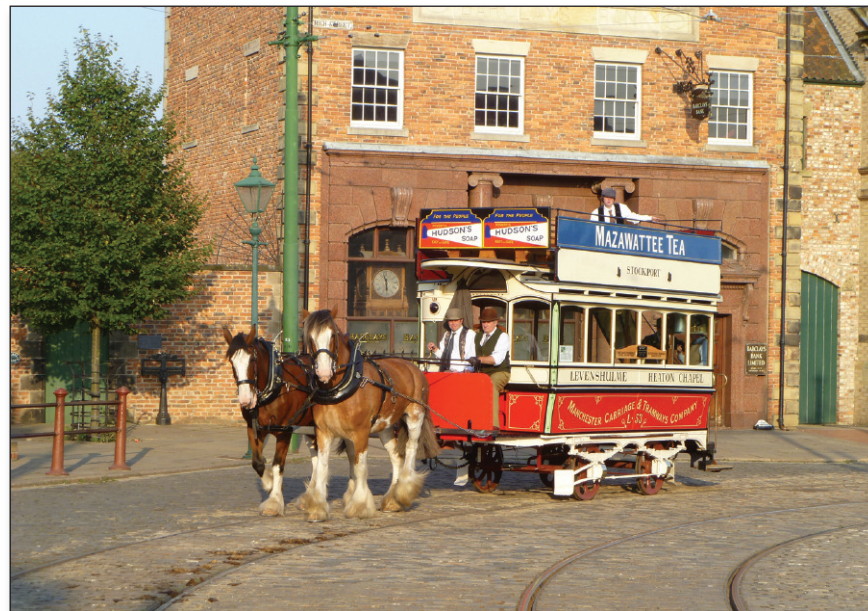
The Heaton Park Tramway's award-winning restored Manchester Carriage and Tramways Company Eades patent reversible horse tram No L53, unique among surviving trams in that it uses the horses' own power to turn the body of the tram round on its underframe when reaching the end of the tracks.
